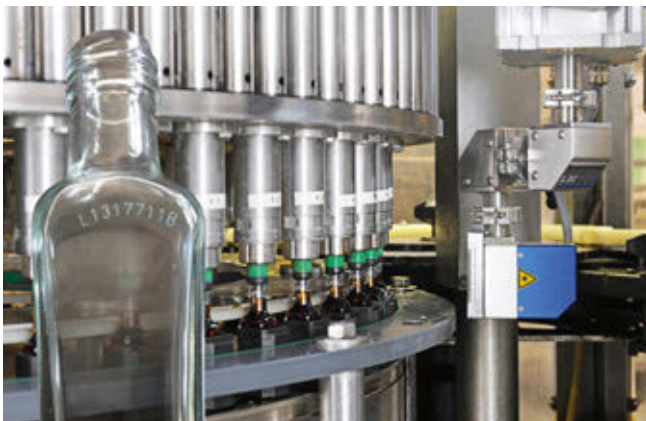
Laser marking of glass
