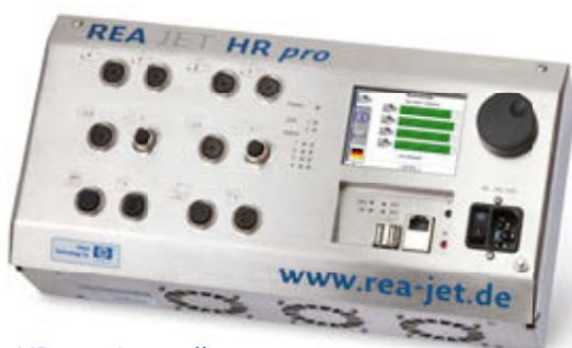
HR pro Controller for control cabinet installation, up to 4 print heads
